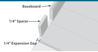
Leave at least 1/4" expansion spaces between flooring and ALL vertical objects (walls, cabinets, pipes, etc.) Large flooring runs may require additional expansion space. Undercut door jambs and casings to provide adequate expansion space. Bamboo Design does not recommend screwing or nailing cabinetry or other permanent fixtures to the flooring.
