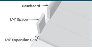
Leave at least 1/4" expansion spaces between flooring and ALL vertical objects (walls, cabinets, pipes, etc.) Large flooring runs may require additional expansion space. Undercut door jambs and casings to provide adequate expansion space. Cali Bamboo® does not recommend screwing or nailing cabinetry or other permanent fixtures to the flooring.
