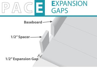
Leave at least 1/2" expansion spaces between flooring and ALL vertical objects (walls, cabinets, pipes, etc.) Large flooring runs may require additional expansion space. For floating floors, use transition moldings between rooms and doorways 3ft. or less. Undercut door jambs and casings to provide adequate expansion space. Do not screw or nail cabinetry or other permanent fixtures to a floating floor.
