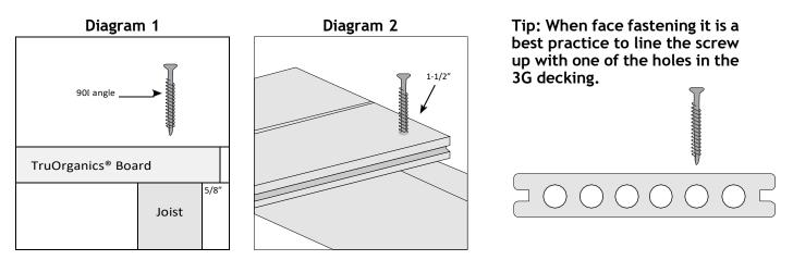
Always use screws designated for use with composite decking material. Test the screws on a scrap piece of board to ensure the screws do not cause the surface of the decking to mushroom or bulge around the head of the screw. If it does cause this issue, change to a different brand of screw.
