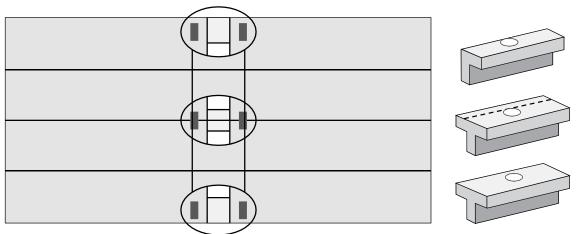
Note: View from above of completed breaker board with T-Clips cut in half.
