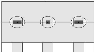
When installing boards we recommend locking the board in the middle to allow for even expansion and contraction to take place on both ends as shown in Diagram 10.
