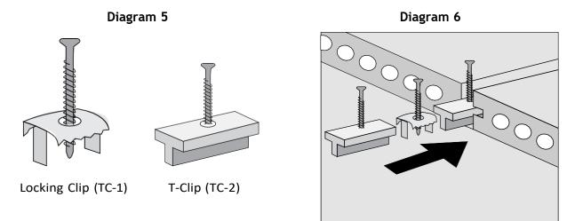
2. After getting all the TC-1 and TC-2 clips into position above each respective joist, begin to fasten them from above as shown in Diagram 6 and 7.
