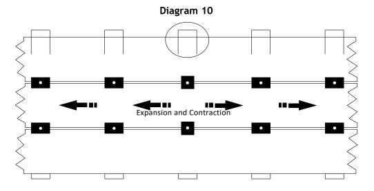
When installing two boards across the deck, locking clips are recommended at the butt joints to help manage proper gapping during expansion and contraction as shown in Diagram 11.
