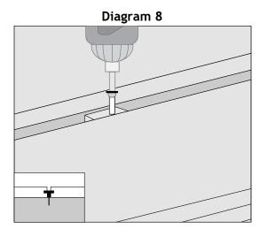
3. The final installed clips should look like Diagram 8.
